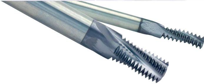
When cutting an internal thread, the linear feed rate needs to be reduced to compensate for the ratio of the tool's cutting diameter to the major diameter being cut. If you do not compensate, the feedrate that the cutting edge sees will be much greater and tool failure will occur. The threadmilling feedrate is equal to:  $(\text{major dia} - \text{cutter diameter}) / \text{major diameter} \times \text{linear feed rate}$
